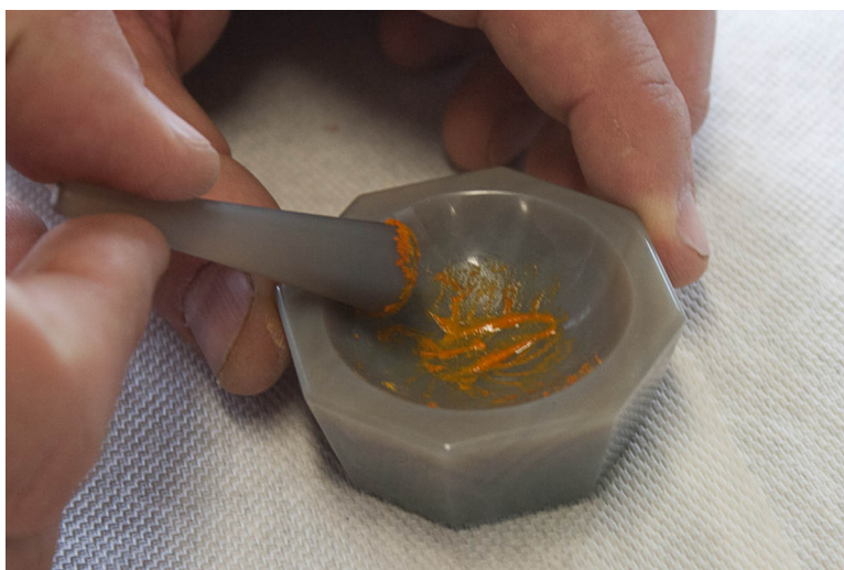
Figure 3.28: Mulling ferrocene into mineral oil with a mortar and pestle.
