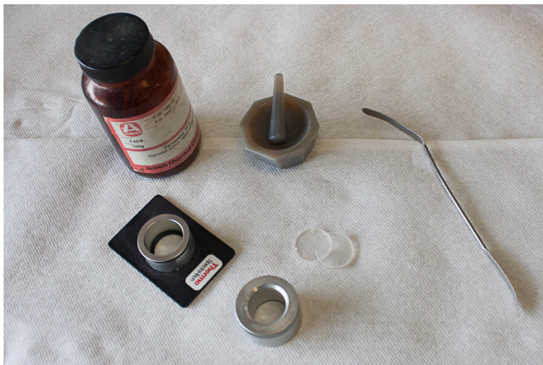
Figure 3.27: In this photograph, the sample, ferrocene, two clean and polished KBr plates, an agate mortar and pestle, a mounting card and a spatula are displayed as the base minimum requirements for preparing a sample though a Nujol mull. Of course, a small bottle of mineral oil is also necessary.
