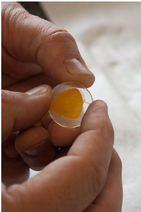
Figure 3.30: Sandwiched KBr plates with a Nujol mull of ferrocene.
