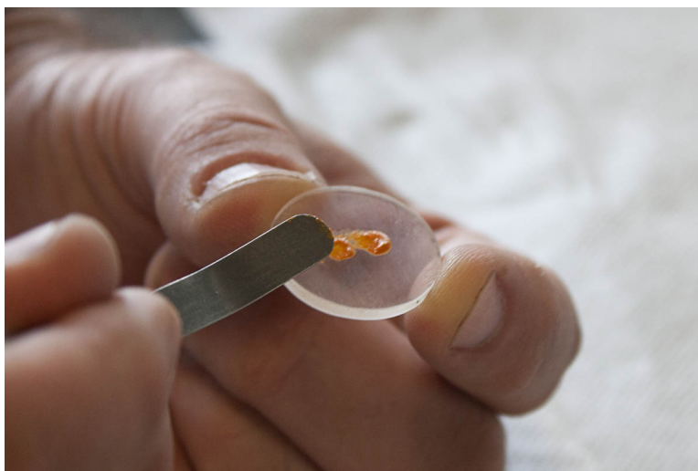
Figure 3.29: The prepared mull from an agate mortar and pestle being applied to a polished KBr plate.
