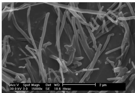
**Figure 2.8:** SEM image of vapor grown carbon nanofibers.
