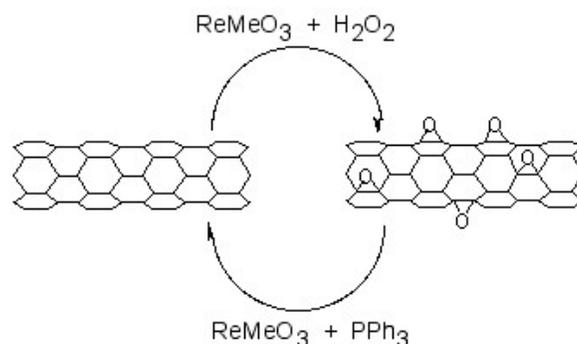
**Figure 2.10:** Catalytic oxidation and de-epoxidation of SWNTs.
