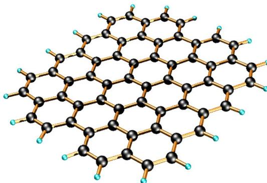
**Figure 2.11:** Idealized structure of a single graphene sheet.
