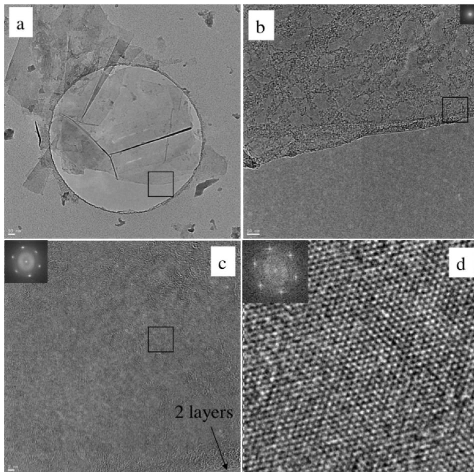
**Figure 2.13:** TEM images of single layer graphene from HOPG dispersion. (a) monolayer and few layer of graphene stacked with smaller flakes; (b) selected edge region from (a), (c) selected area from (b) with FFT inset, (d) HRTEM of boxed region in (c) showing lattice fringes with FFT inset. Adapted from C. E. Hamilton, PhD Thesis, Rice University (2009).
