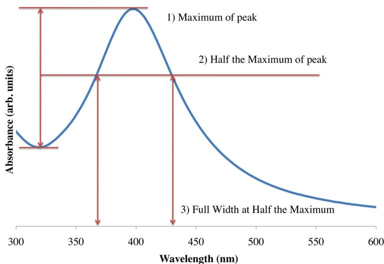
**Figure 2.25:** A plot demonstrating the three steps to obtain the FWHM from a graph of the UV-vis spectrum for the silver nanoparticles.
